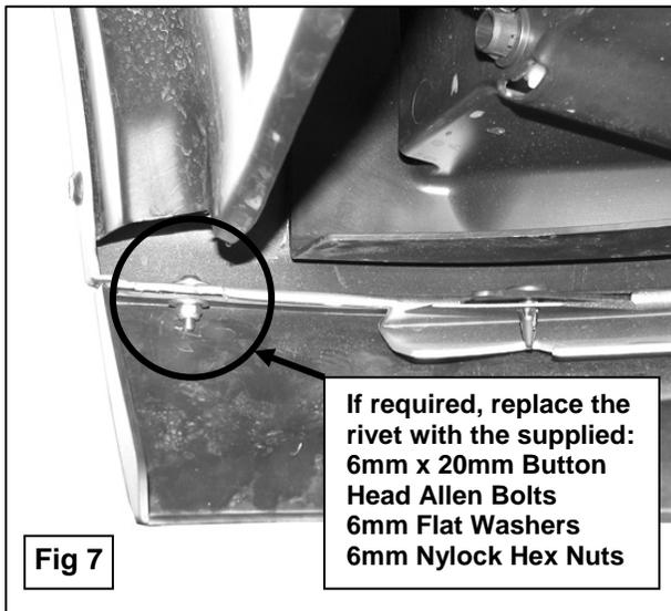
If required, replace the rivet with the supplied:
