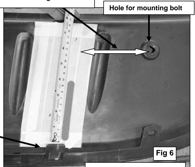
Cut only what is needed to insert bracket through the splash guard. Do not cut through the front edge of the splash guard
