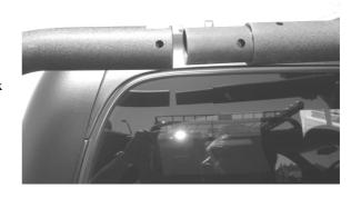
Figure 6 – Uprights installed but not tightened – Important, do not tighten until the cross bars are installed.
