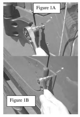
4. Using the supplied front upright 1/4x20 allen bolts and a ¾" flat washer, attach the front upright to the Jeep. You will need a partner to place the factory backing plate (Figure 2) for the lower door hinge in location for you to attach the lower door bolts. (Do not open the door you are working on! Enter from the opposite side). Tighten the bolts for the upright and repeat the process for the opposite side. (Figure 3)
