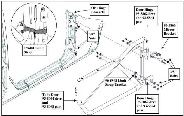
**Step 9:** Carefully close the door and latch it to the door striker. Adjust the door striker if the door won't close properly.
