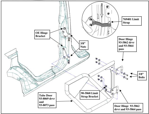
**Step 9:** Carefully adjust the (2) door hinges to level the door on the vehicle.
