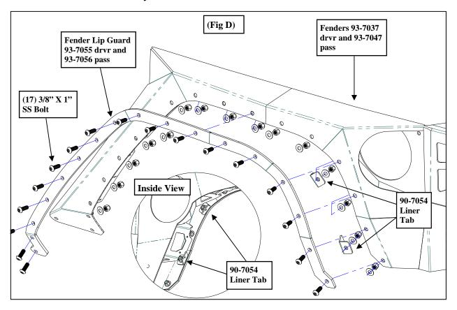
**<u>Step 13</u>**: Remove the clamps and secure the armor fender using the supplied **3/8**" **X 1**" bolts and hardware. Be sure to start all the bolts by hand to avoid cross threading the bolts. Fig. B & C.
