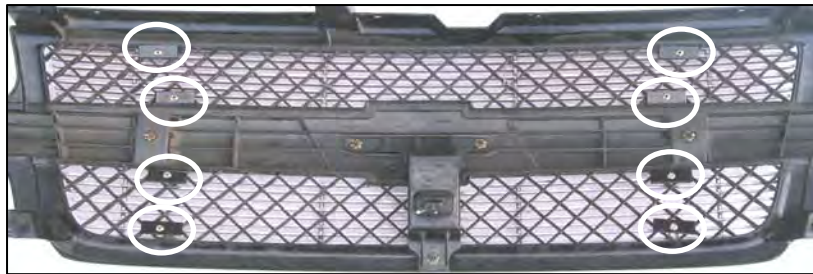
Figure 3 – Rear view of vehicle's shell; top and bottom Billet Grill attached with Metal Brackets and Flange Nuts
