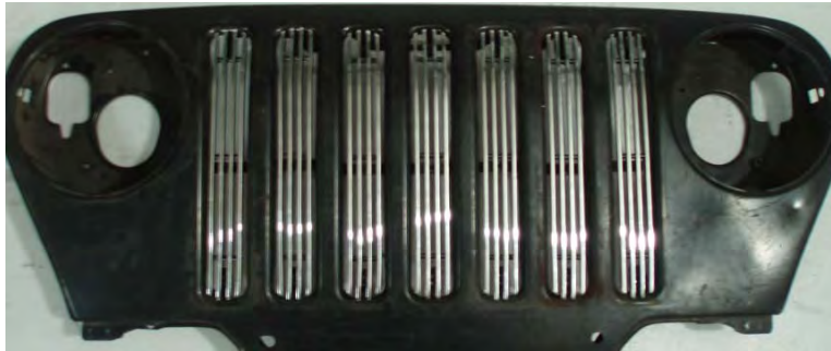
Figure 2 – Front View of positioning lower Billet Grille
