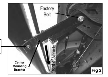
10mm x 25mm Hex Head Bolt 10mm Lock Washer 10mm Flat Washer
