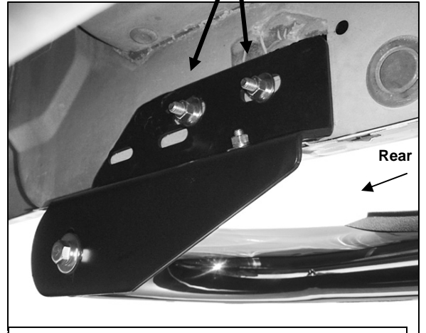
(Fig 4) Rear Mounting Bracket installation (except driver side Mounting Bracket on 97-98 3-door models)
