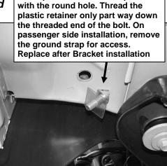
Insert the Nut and Bolt Plate into this square hole and line up the nut
