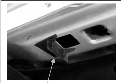
Fig 3. Thin foam adhesive tape. Driver side front
