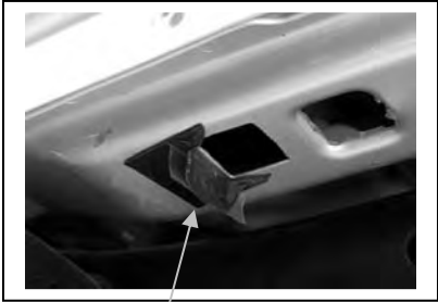
Fig 3. Thin foam adhesive tape. Driver side front
