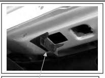
Fig 3. Thin foam adhesive tape. Driver side front
