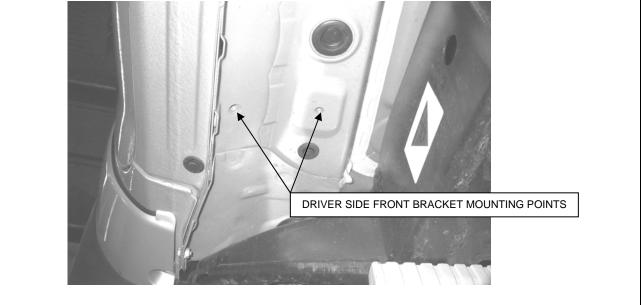
**STEP 2.** This installation uses (3) brackets per side. Begin by installing the driver side front bracket. Locate the (2) threaded holes in the underside body panel.
