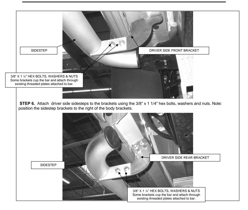
STEP 7. Align the sidestep with the body, and then tighten all bracket and sidestep nuts and bolts.
