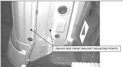
**STEP 2.** This installation uses (2) brackets per side. Begin by installing the driver side front bracket. Locate the (2) threaded holes in the underside body panel.
