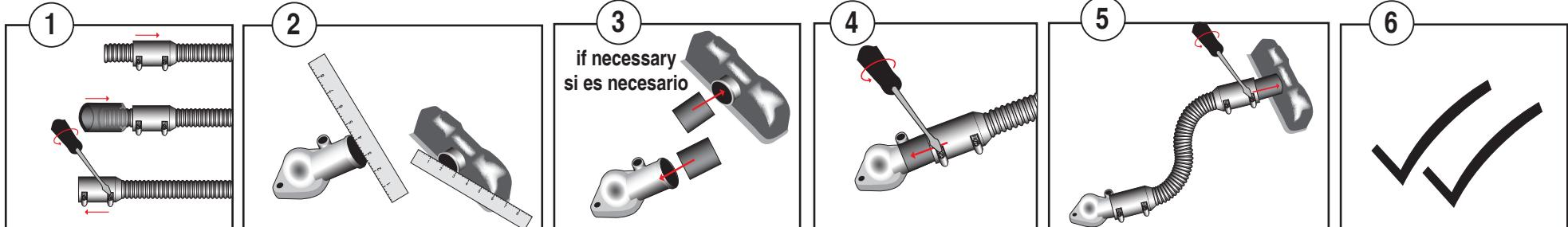
1. Slide clamp section onto the hose above the rubber sealing boot. Position rubber boot halfway onto hose making sure that the narrow inside diameter portion of the boot covers the hose and the wider inside diameter section extends beyond the end of the hose. Slide clamp back to cover the rubber boot and tighten upper clamp to secure clamp to hose. Repeat on the other end.
