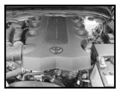
Step 2 Remove the engine cover.
