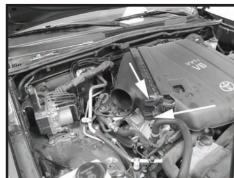
Step 16 Install the gasket inside the base of the air box. Then install the air box cover into the vehicle making sure to use the factory retaining clips to hold the cover in place.
