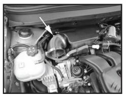
Step 11 Install the 60° coupler and secure the boot in place. Install a second clamp but do not tighten at this time.
