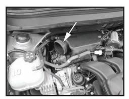
Step 10 Install the throttle body adapter ring onto the plenum.
