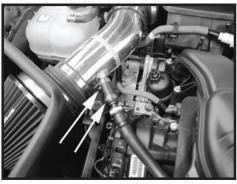
Step 16 Install the supplied vent/barb fitting with the barb side towards the intake tube. Once the fitting is snapped in the factory hose fitting, install the breather hose supplied onto the barbed end of the fitting and connect it to the intake tube. Fasten it securely with the clamps provided.
