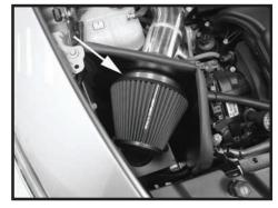
Step 15 Install the filter and fully tighten the clamp.
