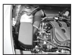
Step 5 Remove the air box assembly by pulling up and out firmly.
