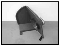
Assemble the heat shield with the tabs placed on the outside of heat shield. Install the rubber bulb seal. Place the velocity stack adapter in the heat shield and install the supplied flex coupler making sure the coupler is pushed completely against the heat shield. Take note of the orientation of the funnel, this may be rotated slightly once the filter is installed in the vehicle. Once the adapter and coupler are tight against the heat shield, tighten the clamp.
