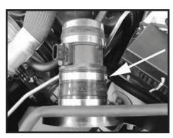
Step 14 Install the MAFS into the reducer coupler on the heat shield. Once in place, tighten the clamp.
