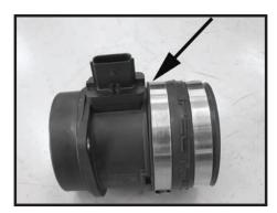
Step 13 Install the 3" coupler on the end of the MAFS. Once in place, tighten the clamp.
