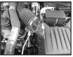
Step 3 Slide the red clip back then disconnect the electrical connector at the Mass Air Flow Sensor (MAFS). Unclip the wiring harness from the air box.
