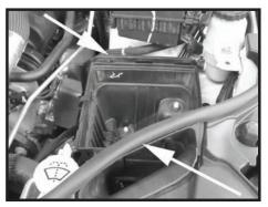
Step 6 Unclip the factory edge trim from the scoop. Remove the lower air box by lifting upwards until the grommets pop out of the locating pins. Unclip the wiring harness from the lower air box and then remove it from the vehicle.
