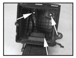
Step 7 Remove two of the factory grommets from the air box. Unclip and remove the factory scoop from the lower air box. These items will be reused in a later step.
