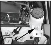
Step 11 Remove the power steering reservoir bolt from the vehicle. This will be reused on Step 12.
