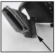
Step 10 Install the scoop into the scoop mount bracket.
