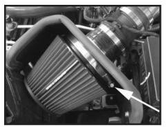
Step 18 Install the filter and fully tighten the clamp.
