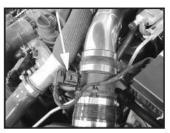
Step 17 Reconnect the MAFS wiring harness. Once bottomed out push the red clip towards the tube to lock in place.
