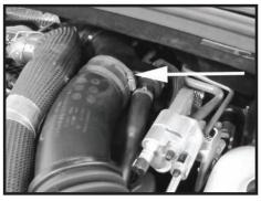
Step 4 Loosen the clamp on the intake tube back by the fire wall.
