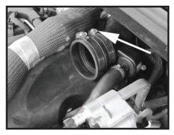
Step 15 Install the reducer coupler onto the factory intake tube. Once in place, tighten the clamp.
