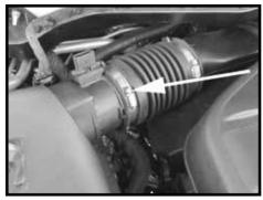
Step 3 Loosen the clamp from the intake tube to the MAFS.
