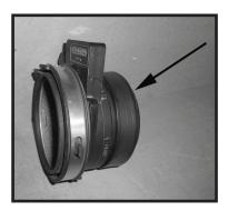
Step 11 Install supplied MAF sensor sleeve over the MAF sensor, making sure that the sleeve is completely bottomed out on the flange.
