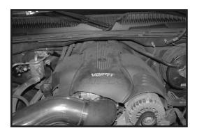
Step 19 Reinstall the engine cover.
