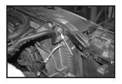
Step 13 Remove bolt from radiator shroud. This will be reused in the next step.
