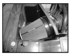
Step 18 Install the filter and fully tighten clamp.
