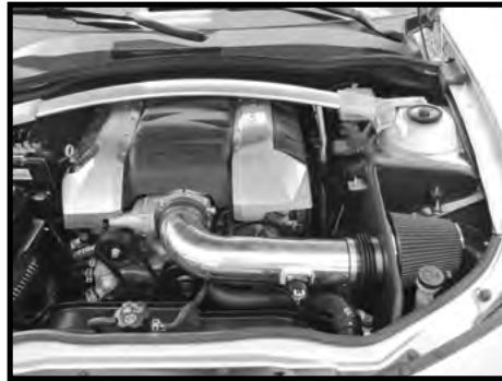
Step 19 Install the engine cover. Make sure that all clamps and hardware are fully tightened. Reconnect the battery cable, start the vehicle and let it warm up. Shut off and inspect the installation once more for any loose clamps, wires, or hardware. Test drive & enjoy! Your installation is now complete. Periodically check all clamps and brackets.
