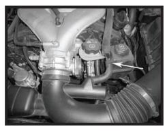
Step 4 Remove the hard PCV line from the rubber 90deg hose by pulling the line firmly out.
