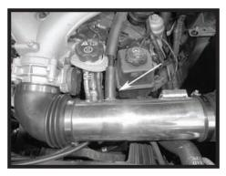
Step 16 Install the vent hose to the intake tube and to the hard PCV line.
