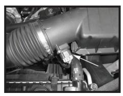
Step 3 Disconnect the electrical connector on the Mass Air Flow Sensor (MAFS).
