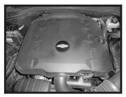
Step 2 Remove oil filler cap and lift the plastic engine cover off. Reinstall the cap to prevent anything from getting inside the engine.
