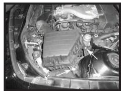
Step 6 Remove the two mounting nuts on the air filter box. Lift then entire air box assembly out of the engine compartment. One of the nuts will be used in **Step 11.**
