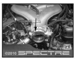
Step 11 Install the throttle body adapter onto the throttle body.
