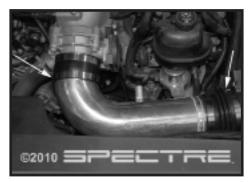
Step 15 Install the intake tube placing the flex coupler onto the MAFS first then placing the other end into the throttle body coupler. Once in place, tighten all clamps.
