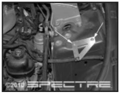
Step 8 Install the heat shield bracket as shown in the image.
