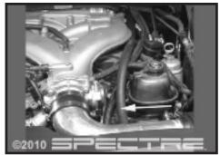
Step 16 Install the new PCV breather line supplied in the kit. Once in place securely fasten with clamps provided.
