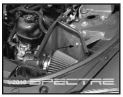
Step 10 Install the heatshield as shown using supplied hardware against the bracket and reinstalling the bolt that was removed in step 9.
