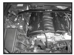
Step 6 '06-'07 models only - Remove the oil fill cap then lift and remove the passenger side engine cover.
