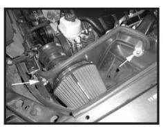
Step 13 Install the heat shield and once in location, fasten securely with the supplied hardware.
