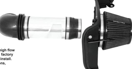
This kit comes with a high flow lifetime hpR filter. It is factory pre-oiled and ready to install. For cleaning instructions, visit our website – www.SpeedBySpectre.com For filter reorders ask at the special order counter of your local parts store or call: 1-909-673-9800
