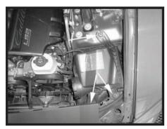
Step 5 Remove the three factory bolts holding the factory air box in place. Remove the air box from the vehicle. For '04-'05 models, skip to Step 9.
