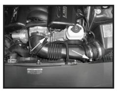
Step 2 Loosen the factory clamp on the throttle body and at the Mass Air Flow Sensor (MAFS).
