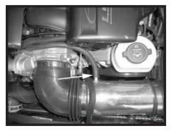
Step 16 Install the new crank case vent hose to the fitting on the intake tube ('06-'07 models). If your vehicle does not have a crank case vent hose, use the supplied vacuum cap to cap off the fitting ('04-'05 models).
