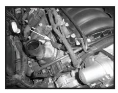
Step 7 '06-'07 models only - Remove the factory crank case vent line from the vehicle.
