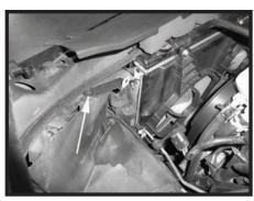
Step 12 Install the heat shield bracket in the vehicle reusing one of the bolts removed in Step 5.
