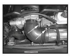
Step 15 Install the flex coupler end over the tube then install the straight end of the coupler over the throttle body and secure the coupler with the supplied clamps.
