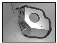
Step 14 Install the engine cover bracket to the heat shield using the supplied hardware. Also install the supplied zip tie into the hole in the heat shield.
