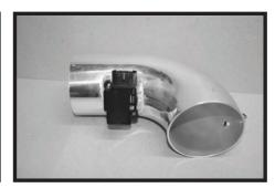
Step 7 Install the MAFS into the aluminum intake tube.
