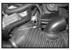
Step 3 Disconnect the PCV breather line from the back of the factory intake tube.
