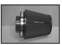
Step 15 Assemble the air filter with the velocity stack adapter and tighten clamp.
