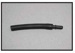
Step21 With the supplied small rubber hose, connect the barbed end of the PCV breather fitting to the hose.
