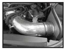
Step 19 Reconnect the mass air flow sensor electrical sensor.
