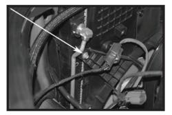
Step 8 Remove the bolt pictured that is supporting the fan shroud.
