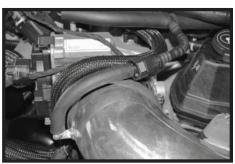
Step 22 Connect the assembled hose from step 29 to the aluminum intake tube and the factory PCV breather line.
