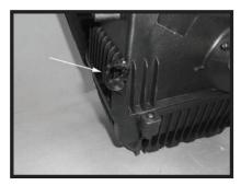
Step 10 Remove the factory hose clip from the factory air box.
