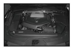
Step 2 Lift and remove engine cover.
