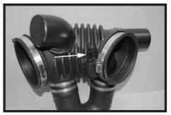
Step 20 Remove the PCV breather fitting from the back of the factory intake tube.
