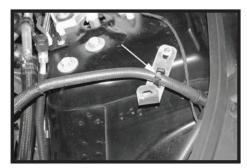
Step 11 Install the heat shield bracket as shown in the image. Install the factory hose clip removed from previous step onto bracket as shown.
