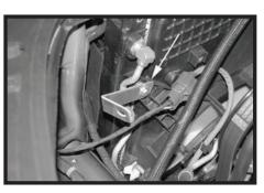
Step 12 Install the heat shield bracket with the supplied spacer between the heatshield bracket and the fan shroud using the supplied hardware.
