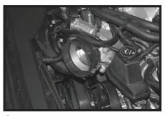
Step 9 Install the 4" coupler onto the throttle body. Tighten the clamp on the throttle side and make sure the intake side clamp is installed but left loose.
