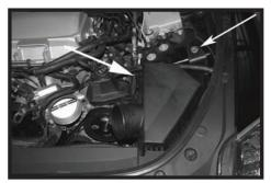
Step 5 Unclip the radiator hose from the clip on the side of the air box. Remove the bolt on the air box and then lift the air box assembly up and out of the engine bay.
