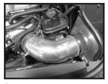
Step 18 Install the intake tube into the coupler on the heat shield and then into the coupler on the throttle body. Tighten all clamps.
