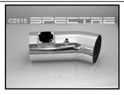
Step 10 Install the mass air flow sensor into the intake tube and secure it using the two supplied m4 Phillips screws.
