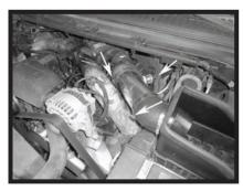
Step 10 Install the Spectre Performance intake tube into the flex coupler first then into the angled coupler with the filter minder closer to the turbo. Once the tube is in position and the filter minder is facing the firewall, tighten the clamps. If you have an electronic filter minder, reconnect the factory wire harness clip.
