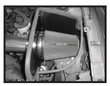
Step 17 Install the filter and fully tighten the clamp.
