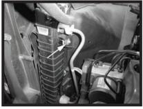
Step 10 Remove the bolt holding the radiator shroud. This will be reused in Step 12.
