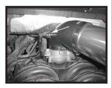
Step 16 Reconnect the factory PCV hose to the fitting on the 90° coupler.
