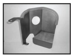
Step 7 Install bulb seal around edges of heat shield as shown.
