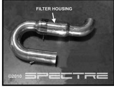
Insert air filter into the short intake tube (with the filter housing) until the lip of the filter is in contact with the edge of the tube. Install the collar clamp boot halfway over the filter housing and position the collar clamp over the boot. Insert the long tube into the boot, positioning it as shown. Snug up the clamp, but do not fully tighten as you will need to rotate the tubes to position them in a future step.
