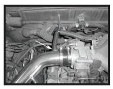
Step 14 Using the 5/8" hose and the 90° fitting, reconnect the vent line to the intake tube as shown.
