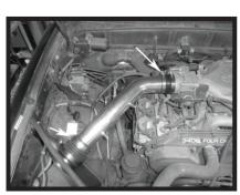
Step 12 Install the intake tube as shown and once in position tighten the clamps.
