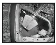
Step 16 Install the filter and fully tighten the clamp.
