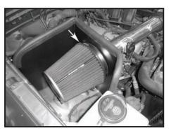
Step 16 Install air filter with the supplied clamp and fully tighten.
