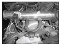
Step 14 Connect the mass air flow sensor connector and the vent hose.
