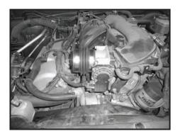
Step 12 Install the flex boot on throttle body and secure the boot in place. Install a second clamp but do not tighten at this time.
