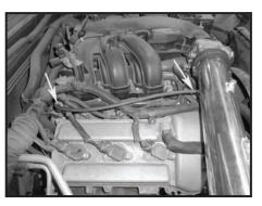
Step 15 Install the supplied vacuum hose from the vacuum fitting to the fuel regulator.
