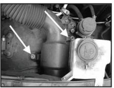
Step 6 Remove the two screws securing the resonator.
