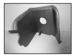
Step 9 Install the rubber bulb seal on the heat shield.
