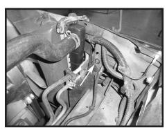
Step 5 Remove the bolt from the front core support of the vehicle.
