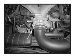
Step 5 Loosen the clamp at the throttle body.
