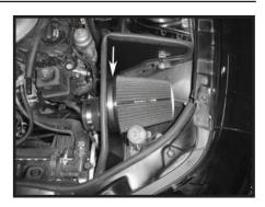
Step 12 Install the filter on the velocity stack adapter and fasten it securely.
