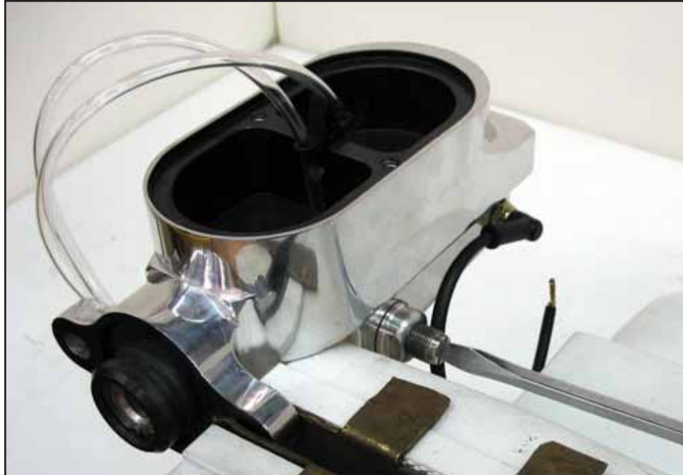
The proportioning valve will be adjusted using a screwdriver. Clockwise will increase brake pressure and counter-clockwise will decrease pressure
