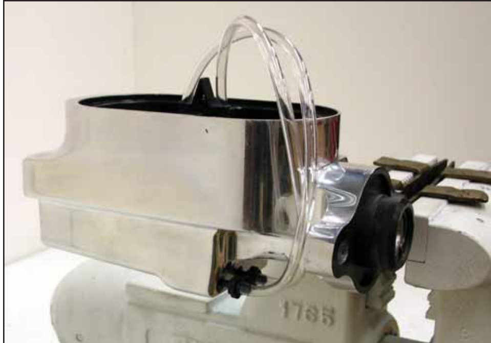
Install bench bleeding kit into master cylinder and fill bowls with new brake fluid
