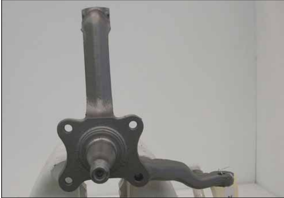
Factory front knuckle with all drum brake parts removed
