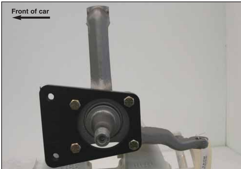
Install base caliper mounting bracket onto spindle and secure with 3/8" bolts and flange nuts supplied. Torque to 35-40 ft/lbs.
