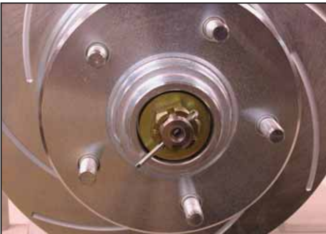
Slide the rotor into place on the spindle, followed by the outer bearing, washer, & nut. After torquing the nut, install the cotter pin
