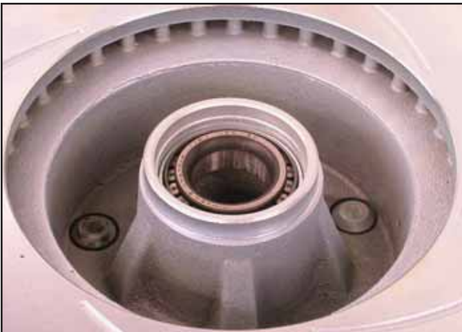
Install the greased inner bearing into the back of the rotor
