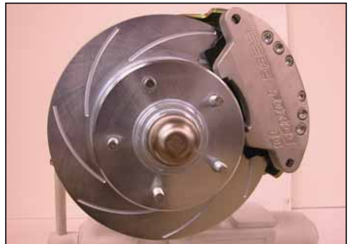
Slide the caliper into position over the rotor and install the slider bolts. Torque to 25 ft/lbs. Spin the rotor by hand to be sure rotor spins freely
