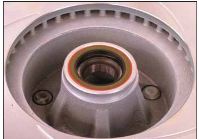
Install the grease seal into the back of the rotor
