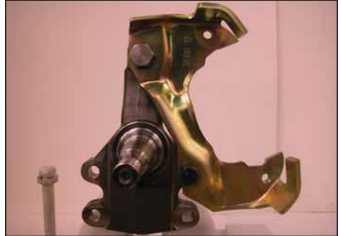
Install the caliper mounting bracket and secure with supplied 5/8" x 1" and 1/2" x 2" bolts
