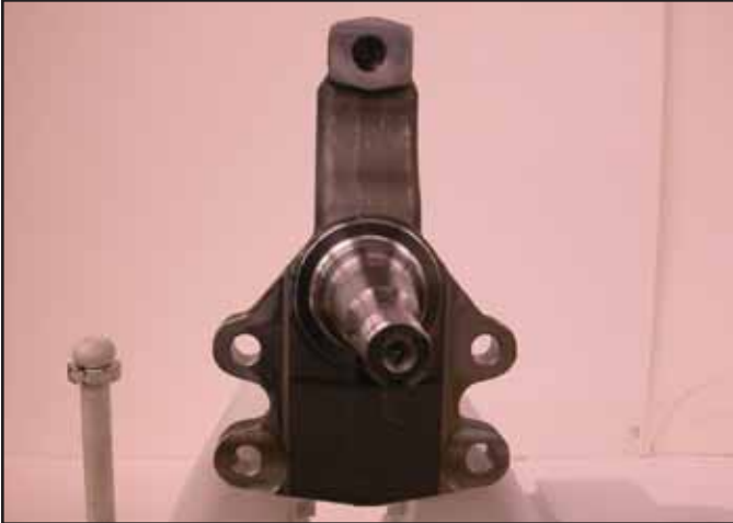
SSBC 2" drop spindles supplied with kit
