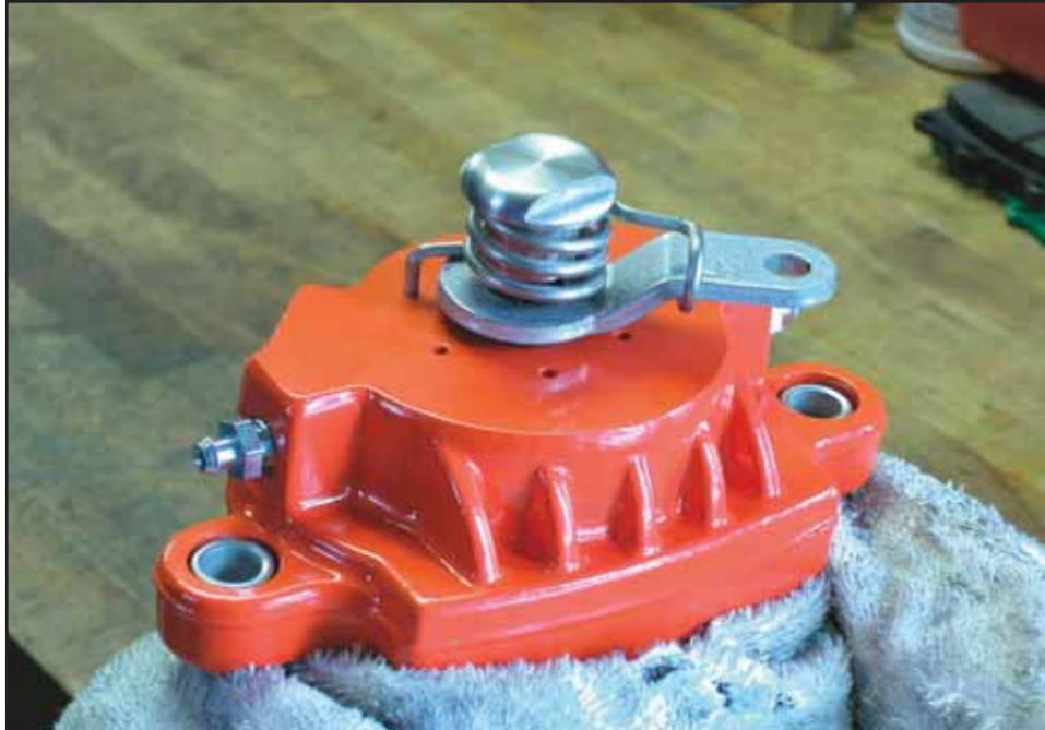
Photo 1: For some applications, it may be necessary to change the position of the parking brake lever to allow connection of the brake cables.
