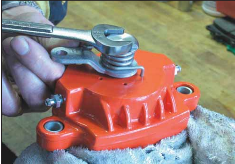
Photo 7: Tighten the retaining nut with a 3/4" open end wrench while holding the parking brake lever.
