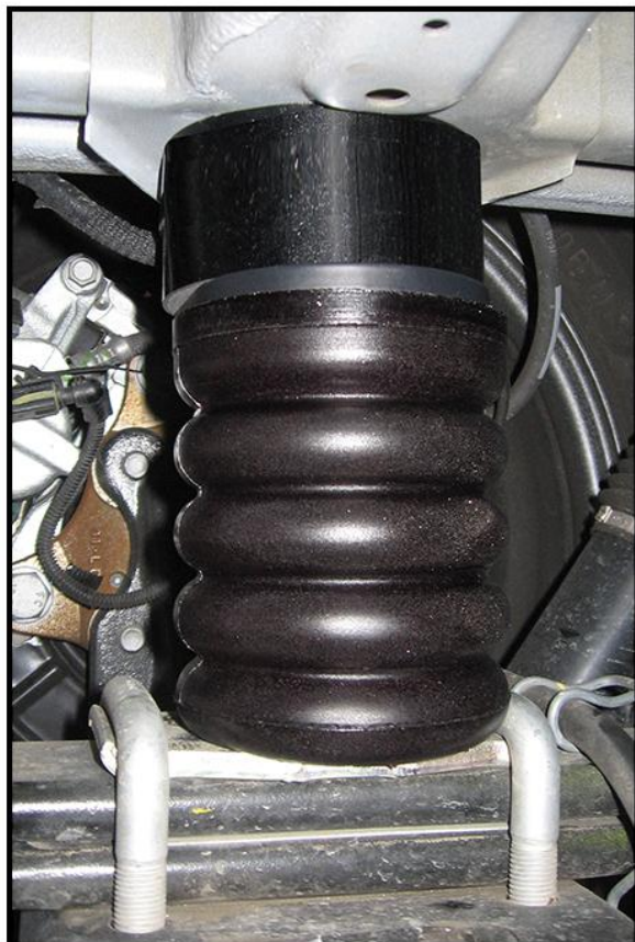
Rear SumoSpring SSR-304-47 Installed
