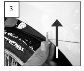
Now the splash shields below the engine must be removed. Note how they interlock; they will need to be re-installed the same way. Remove the nine 7mm bolts along the Bottom. There are two 10mm bolts in the center of this splash shield that must also be removed.
