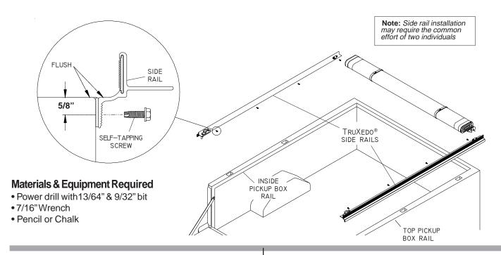
STEP 1: TruXedo® side rails have four pre-punched mounting holes. Hold side rails against front of box, keeping offset portion of rail flush with top rail of box. Chalk mark locations of four holes on inside of pickup box, using mounting holes as guides.
