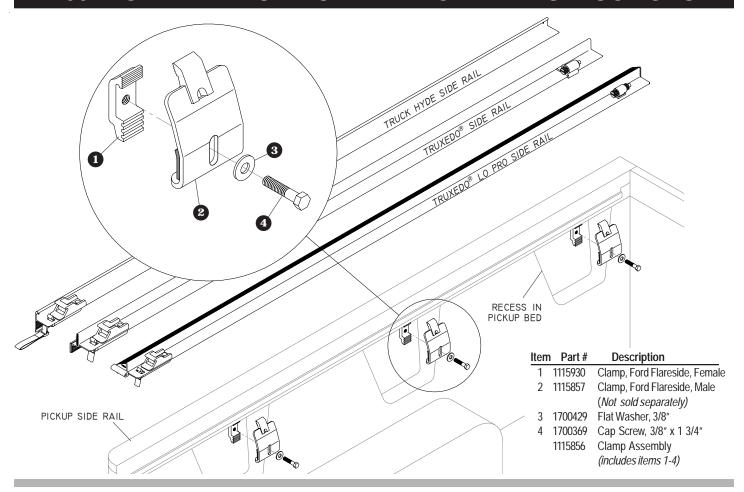
STEP 1: Align clamp assemblies along pickup side rails, centered in recesses.
