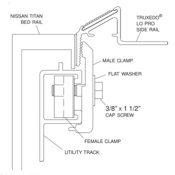
**STEP 4:** Tighten clamps securely.
