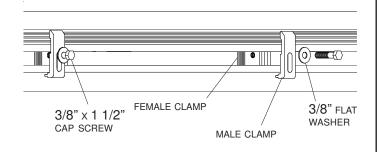
STEP 3: Install TruXedo® side rails, wedging rails between male clamp and bed rail.
