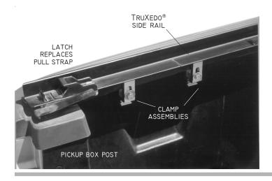
**STEP 3:** Attach two clamp assemblies at rear of side rail in recess of pickup box. Side rail is notched to fit on top of pickup box post.
