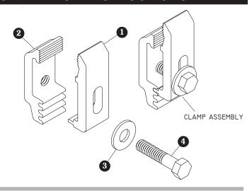
**STEP 1:** Position clamps 9" and 36" from front of box; and 8" and 17" from tailgate (four clamps per side rail).
