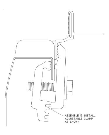
**STEP 4:** Align side rails 1/4" from tailgate, flush with box rail and level with each other. Tighten clamp assemblies (see owner's manual).
