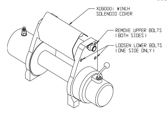
• If the winch has a separate control pack with a black plastic cover, remove the plastic cover being careful not to strain the internal wiring. Replace the cables as described above. Reinstall the cover.
