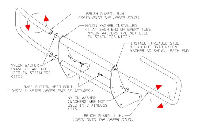
2. The brush guards are then rotated onto the studs as shown. To obtain clearance to rotate the brush guard, it is usually necessary to tilt the Trans4mer Kit forward. To do this, loosen the lower fastener, remove the upper fasteners and tilt as required.
